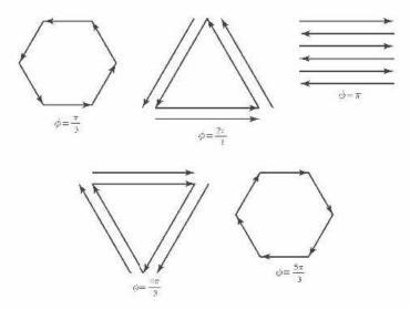
**36.61:** a) For the maxima to occur for N slits, the sum of all the phase differences between the slits must add to zero (the phasor diagram closes on itself). This requires that, adding up all the relative phase shifts,  $N\phi = 2\pi m$ , for some integer m. Therefore
